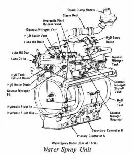
Each WSB provides an expendable heat sink for the orbiter hydraulic system's fluid and APU lube oil system on the ground, during the boost phase, orbital checkout, deorbit, and entry through landing and rollout. The core of each WSB is the stainless-steel, crimped-tube bundle oil cooler. The oil cooler of each WSB consists of a hydraulic fluid section and an APU lube oil section. The hydraulic fluid and APU lube oil flow through their respective sections of the tube bundle oil cooler.
