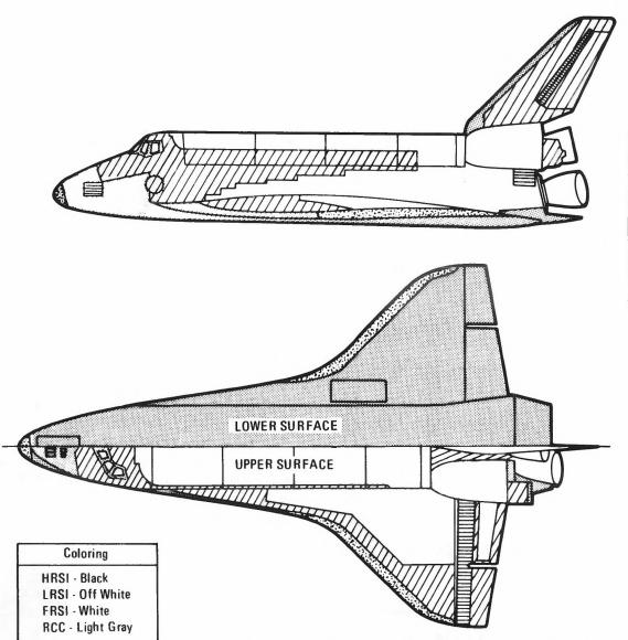
Thermal Protection System, Orbiter 102
