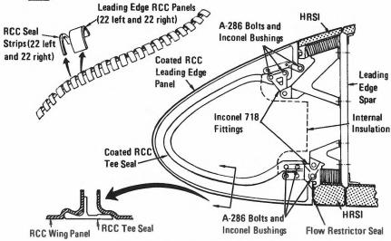
RCC Wing Lead Edge, Orbiter 102 and Possibly Some of Orbiter 099
