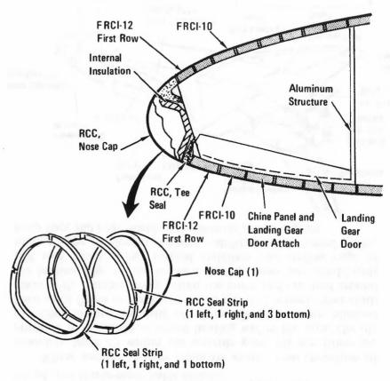
RCC Nose Cap, Possibly Some of Orbiter 099, Orbiter 103 and Subsequent
