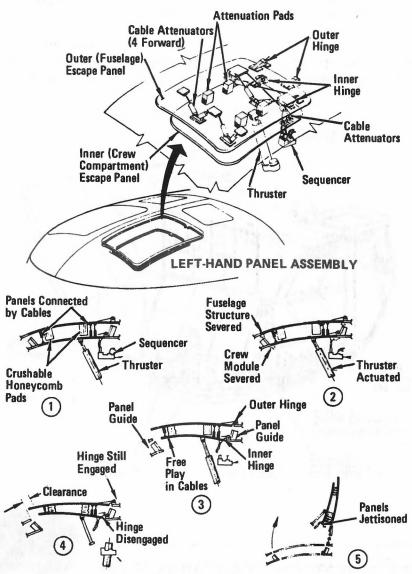
Overhead Ejection Panels - Development Flight Tests
