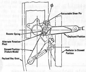
Payload Bay Door, Deployable Radiator Stowed
