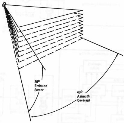
MSBLS Elevation Coverage and Pulse Coding
