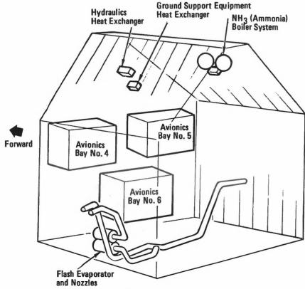
Aft Fuselage ECLSS Components
