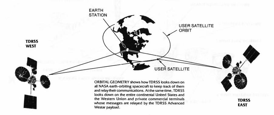
Tracking and Data Relay Satellite System
