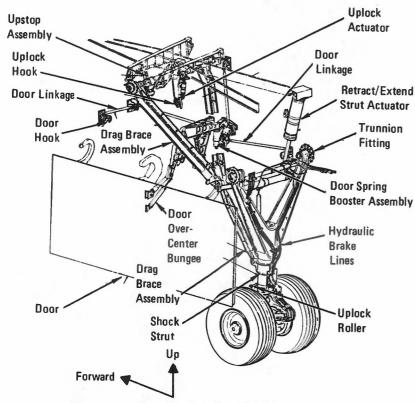
Main Landing Gear Deployed
