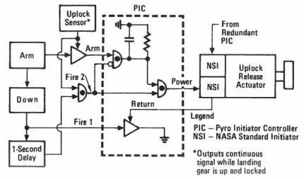
Uplock Release and Pyro Actuator Circuit (Simplified)
