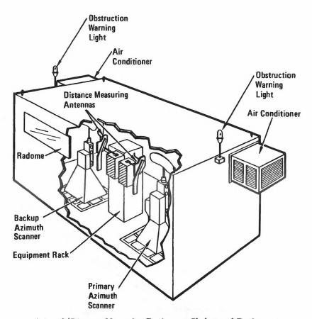
Azimuth/Distance Measuring Equipment Shelter and Equipment
