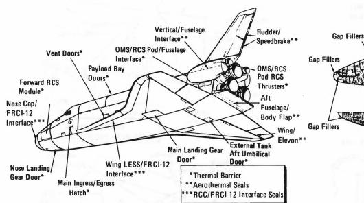
Thermal Barriers, Orbiter 099 and Subsequent Orbiters
