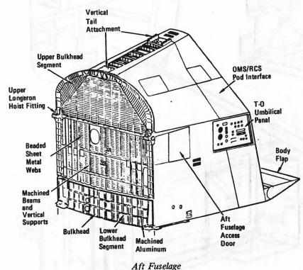
loading and support constraints. Certain system components, such as the avionics shelves, are shock-mounted to the secondary structure. The secondary structure includes support provisions for the auxiliary power units, hydraulics, ammonia boiler, flash evaporator, and electrical wire runs.
