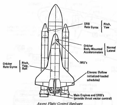
An electrical voltage proportional to the angular deflection about the output axis and representing vehicle rate about the input axis, is generated and sent through the flight aft multiplexer/demultiplexers to the computers and RGA subsystem operating program (SOP). Selected rates are then sent to the ADI rate needles. The data is also sent to the display electronic unit CRT's.
