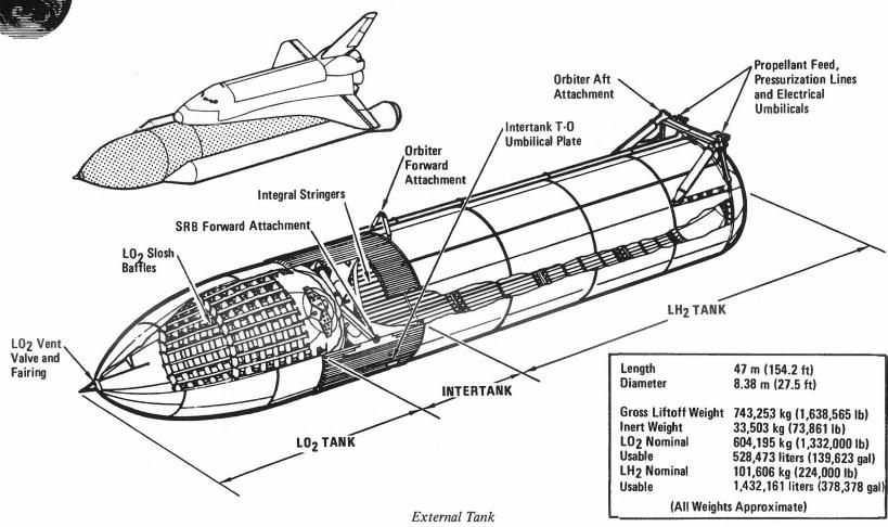
Electrical signals and controls between the orbiter and the two solid-rocket boosters also are routed through those umbilicals.
