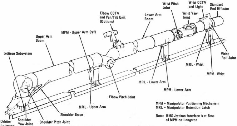
Mechanical Arm - Stowed Position and General Arrangement
