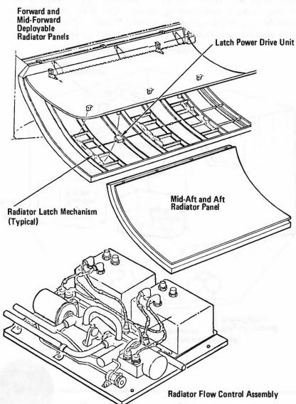
Radiators and Radiator Flow Control Assembly
