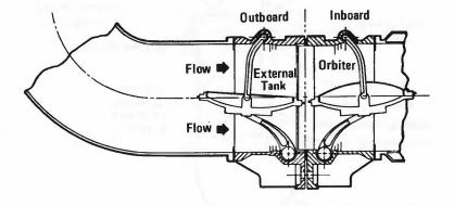
External Tank-Orbiter Disconnect Valves
