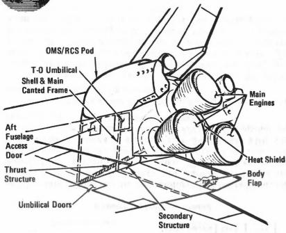
Aft Fuselage Structure
