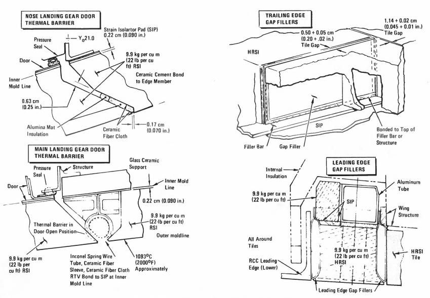
Typical TPS Gap Fillers and Thermal Barriers, Orbiter 102
