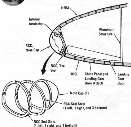
RCC Nose Cap, Orbiter 102 and Possibly Some Orbiter 099 addition, it prevents the direct flow of hot boundary layer gases into the wing leading edge cavity during entry. The "tee" seals are constructed of RCC.
