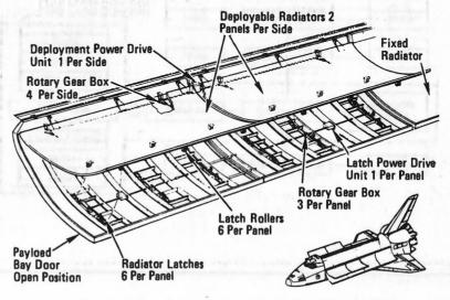
Payload Bay Door, Deployable Radiator Mechanism
