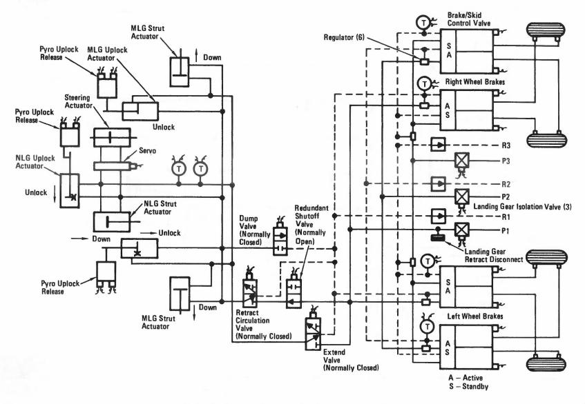
Hydraulic Actuator System - Landing Gear and Brake
