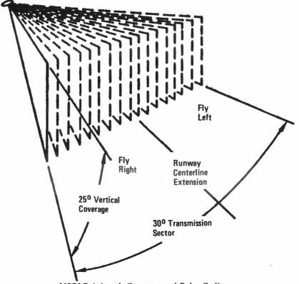
MSBLS Azimuth Coverage and Pulse Coding
