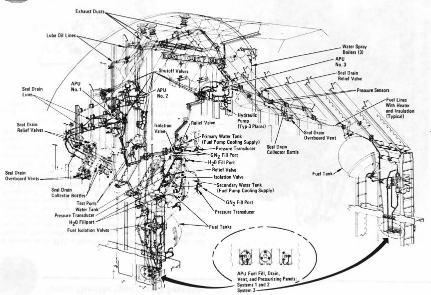
Auxiliary Power Unit/Water Boilers
