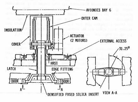
Orbiter/External Tank Umbilical Closeout Doors - Centerline Latch
