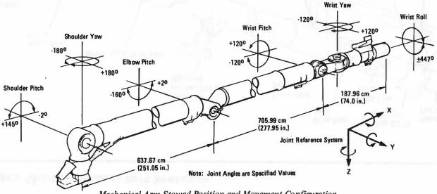
Mechanical Arm-Stowed Position and Movement Configuration
