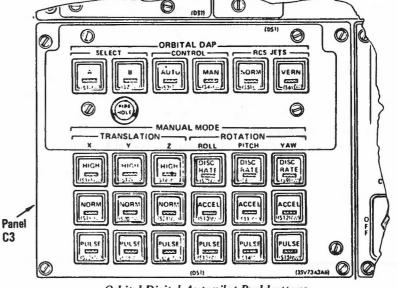
Orbital Digital Autopilot Pushbuttons
