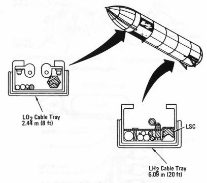
External Tank Range Safety System Linear Shaped Changes
