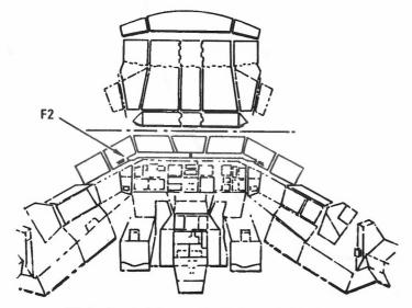
Flight Control System Pushbutton Indicators
