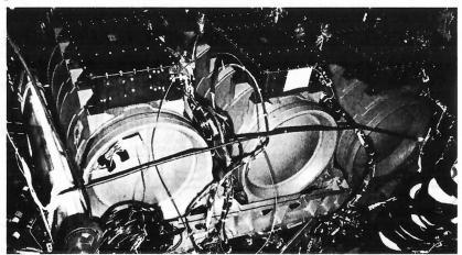
Water Spray Boilers in Aft Fuselage
