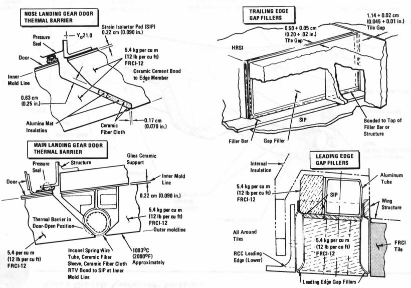
Typical TPS Gap Fillers and Thermal Barriers, Orbiter 099 and Subsequent Orbiters
