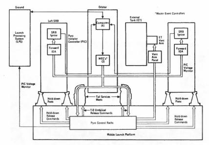
Solid Rocket Ignition, Hold-Down Release, and Umbilical Retract Commands
