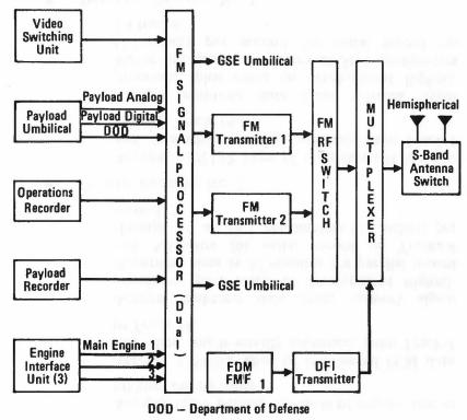
Frequency Modulation Signal Processor
