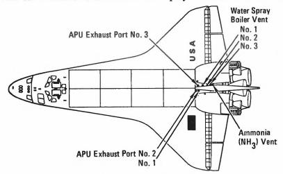
APU Exhaust and Water Boiler Vent
