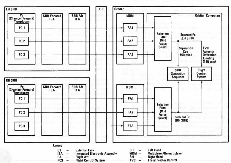
Solid Rocket Motor Chamber Pressure Data Flow
