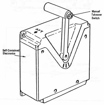
Speed Brake Thrust Control
