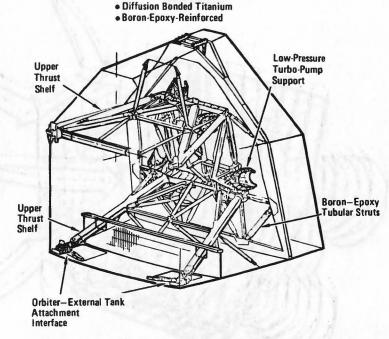
Aft Fuselage Internal Structure
