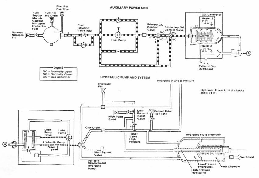
Auxiliary Power Unit and Hydraulic Pump System
