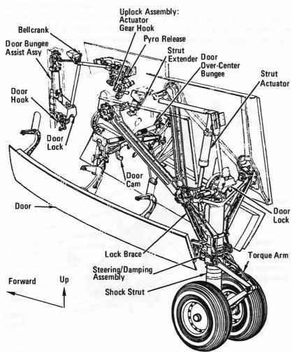
Nose Landing Gear Deployed
