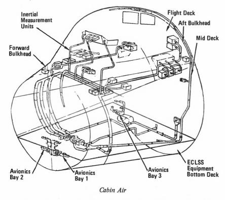
The crew module cabin contains five air loops: the cabin, three avionics bays and the inertial measurement unit cooling loop. The crew module cabin atmosphere is drawn through the cabin through a 300-micron filter by one of two cabin fans located downstream of the filter.
