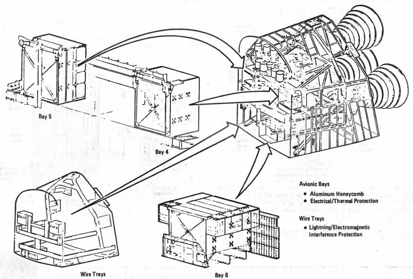
Aft Fuselage Avionics Provisions
