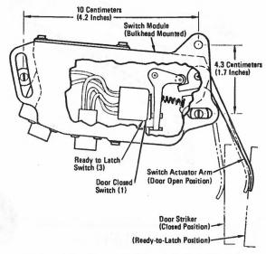
Payload Bay Doors Bulkhead Switch Module
