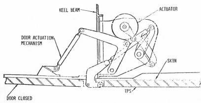
Orbiter/External Tank Umbilical Closeout Doors — Hinge/Actuation System
