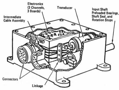
Rudder Pedal Transducer Assembly
