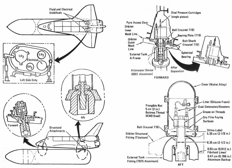
Orbiter - External Tank Separation System
