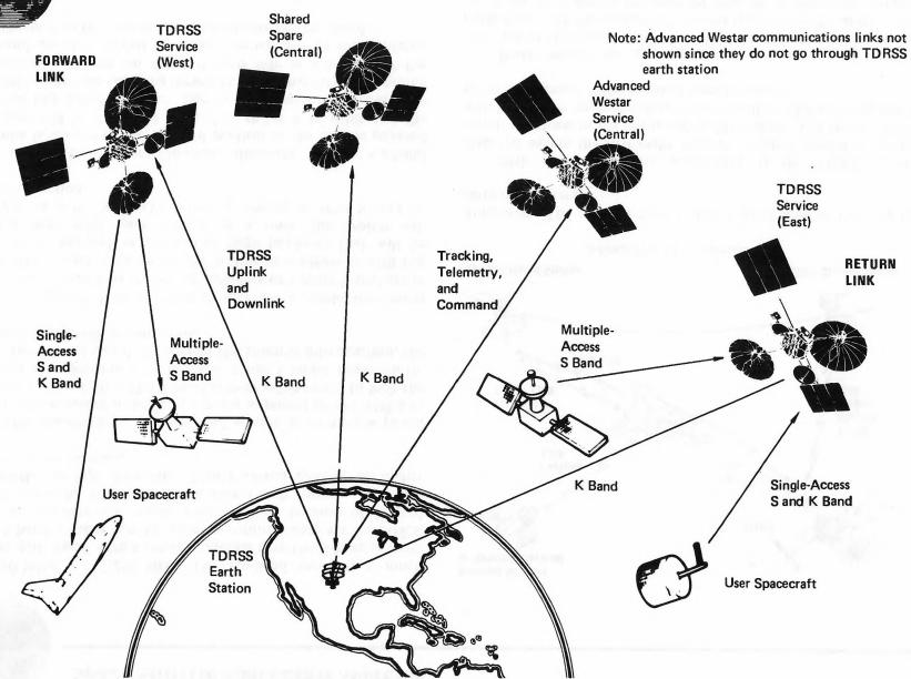
Linking Four Identical and Interchangeable Satellites With Earth Station
