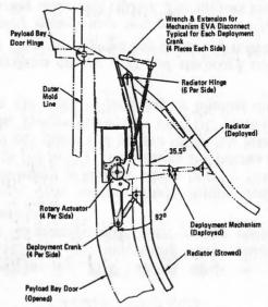
Payload Bay Door, Deployable Radiator Deployed
