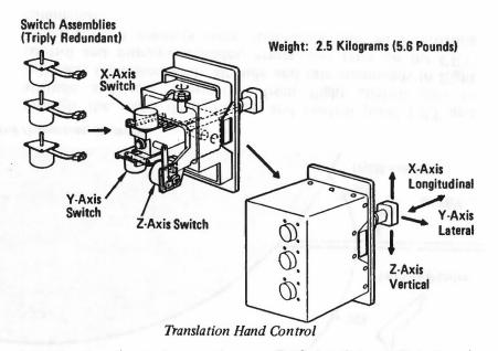
jet selection logic for continuous RCS jet firings. Rotational commands may be sent simultaneously with translation commands within the limits of the RCS jet selection logic; if both plus X and minus Z translations are commanded simultaneously, plus X translation is given priority.
