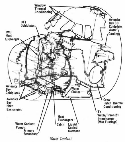
plate and into the  $H_2O$ , which carries the heat away from the electronic unit. Coldplates mounted on the shelves in the avionics bays are connected in a series – parallel arrangement with respect to the  $H_2O$  flow.
