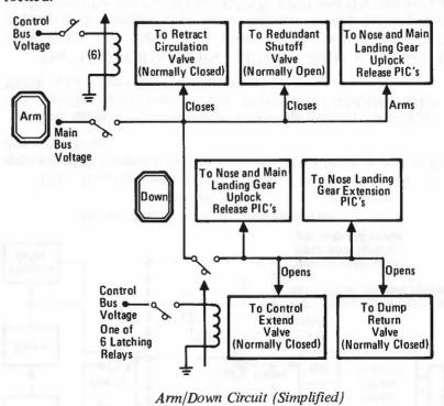
Landing gear deployment is initiated when the CDR or PLT depresses the guarded ARM pushbutton switch/light indicator, then the guarded DN pushbutton switch/light indicator. This is accomplished at least 15 seconds prior to predicted touchdown and at a speed no greater than 300 knots (345 mph).
