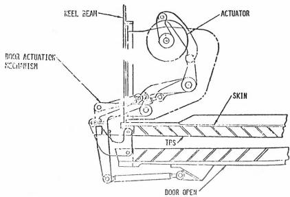
Orbiter/External Tank Umbilical Closeout Doors – Hinge/Actuation System
