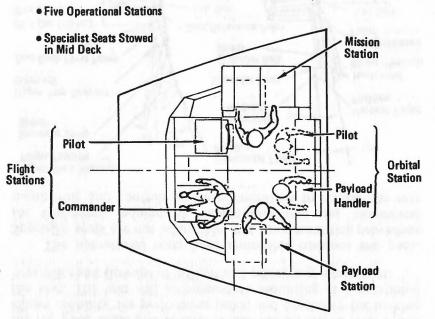
Flight Deck Station - Orbital Operations
