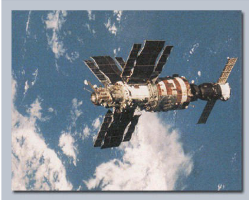
The Salyut-7 orbital station (left) with the docked Soyuz T spacecraft (right) in flight
