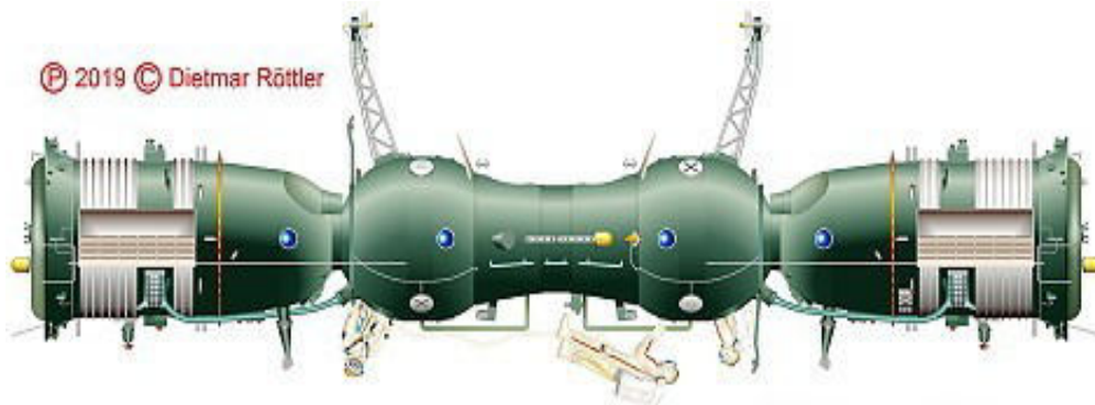
Docking Configuration of SOYUZ 4 and SOYUZ 5
