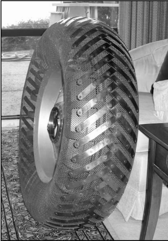
The LRV tire showing the woven piano wire and titanium chevron treads.
