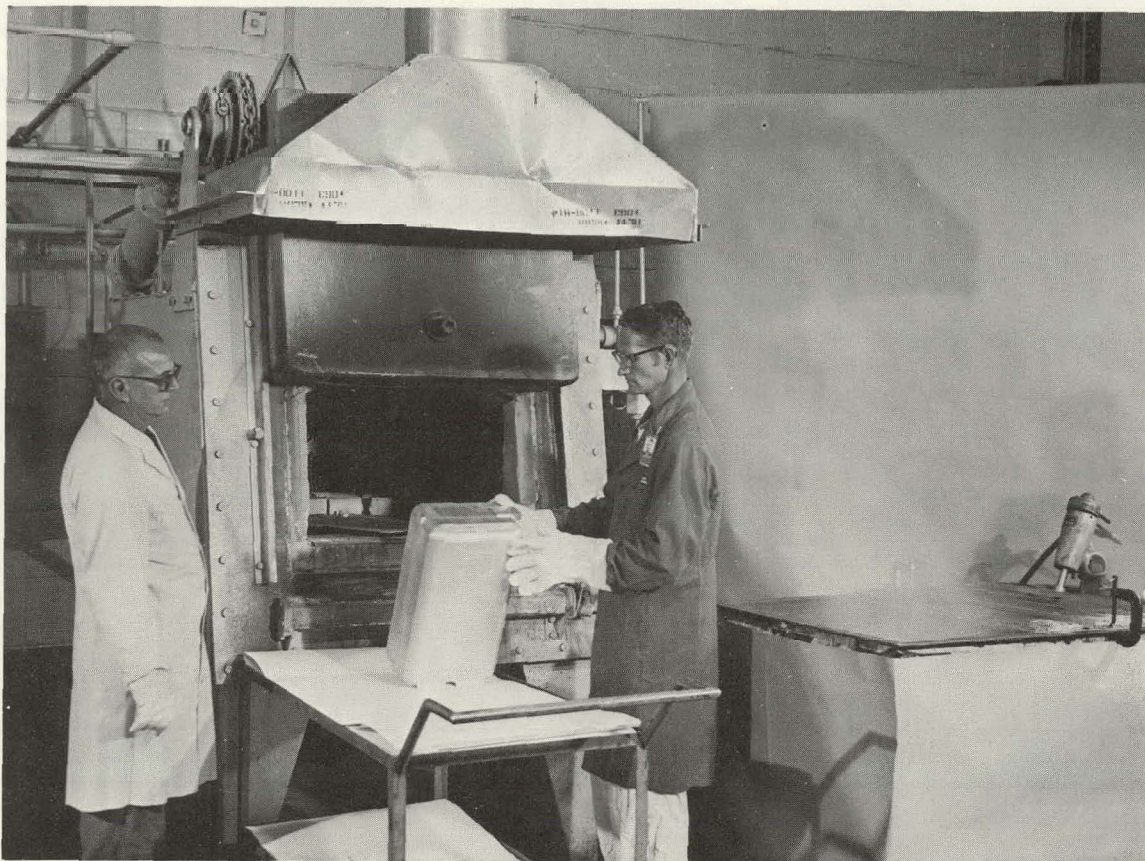
Figure 19. HEAT-TREAT FURNACE WITH ITS WATER-QUENCHING TANK.
