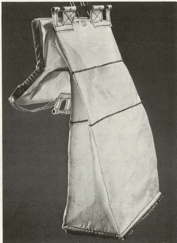
Figure 30. SAMPLE COLLECTION BAG MADE FROM TEFLON FILM AND TEFLON CLOTH.
