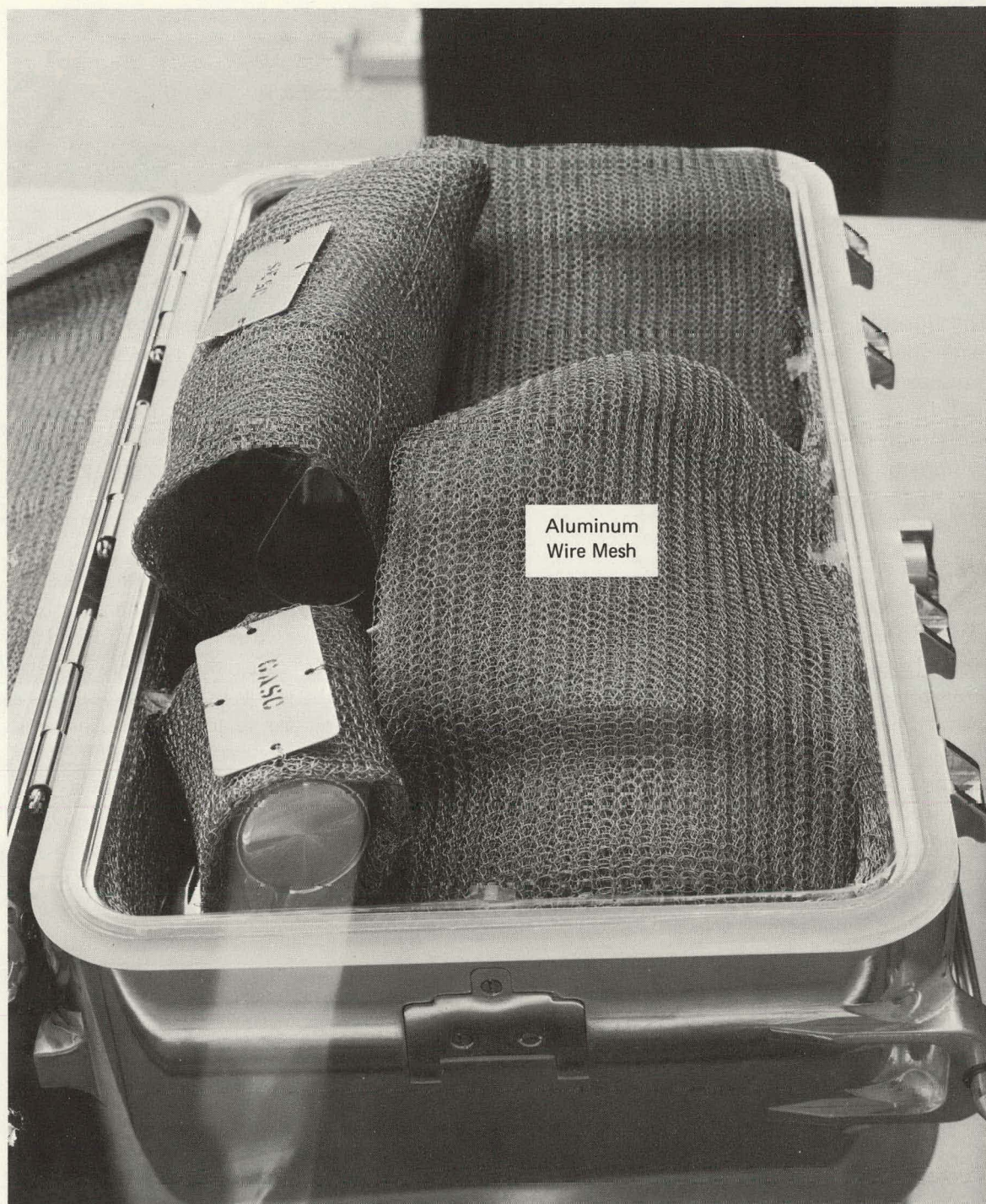
Figure 28. VIEW OF ONE APOLLO LUNAR SAMPLE RETURN CONTAINER FOR THE APOLLO 13 MISSION, SHOWING THE SPECIAL ENVIRONMENTAL SAMPLE CONTAINER AND GAS ANALYSIS SAMPLE CONTAINER PACKED IN THEIR TRANSLUNAR CONFIGURATION.
