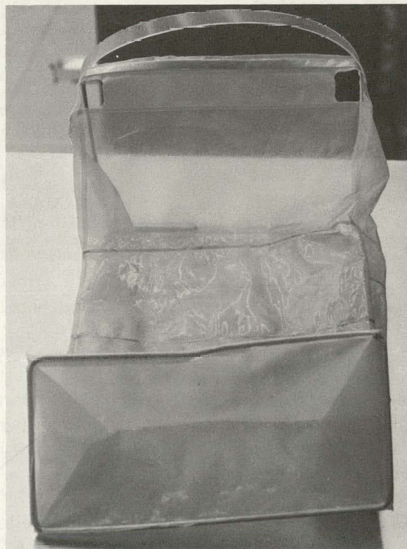
Figure 29. ORIGINAL SAMPLE COLLECTION BAG MADE FROM TEFLON FILM.
