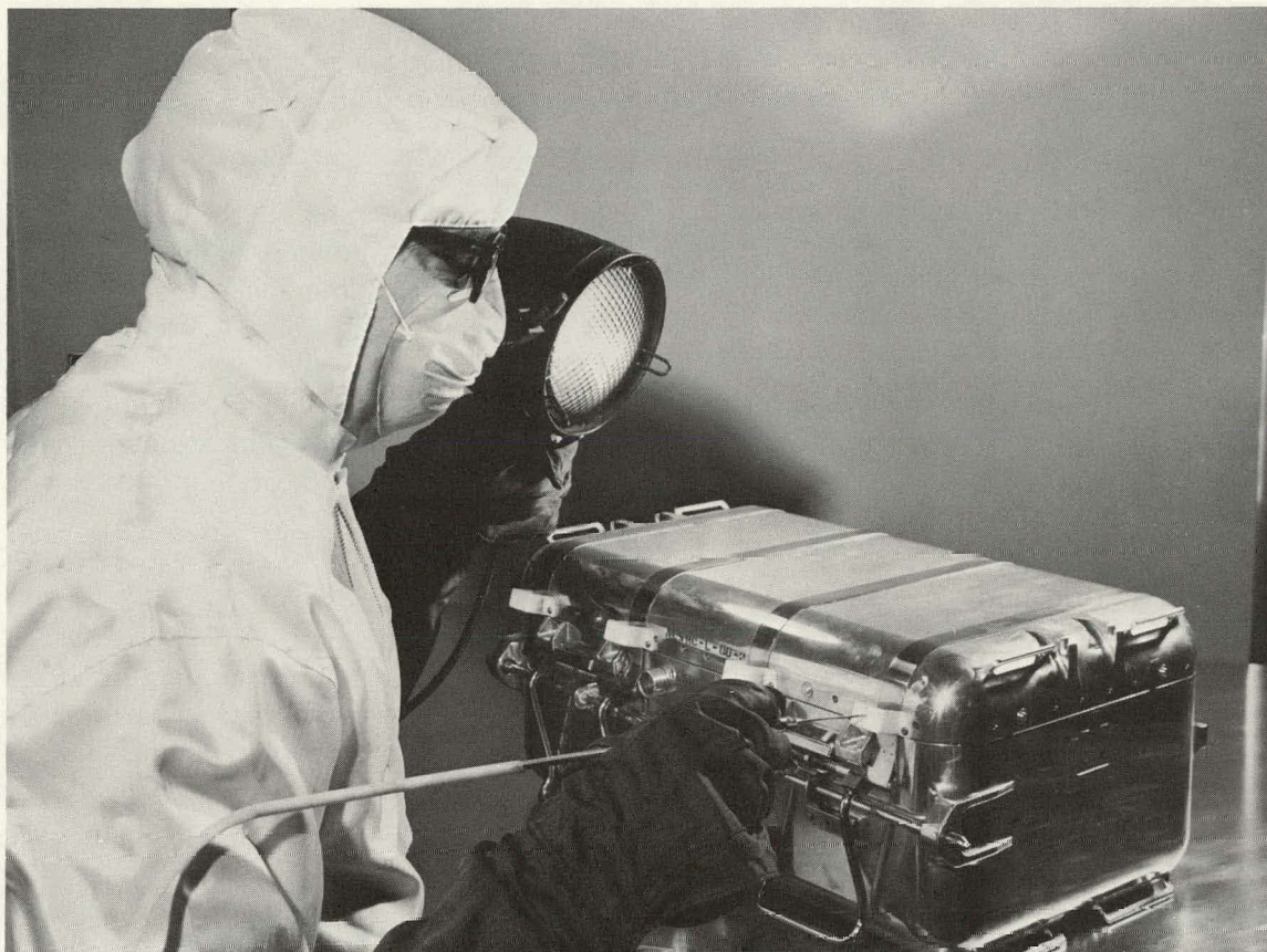
Figure 53. ULTRAVIOLET INSPECTION AND VACUUM REMOVAL OF LINT.
