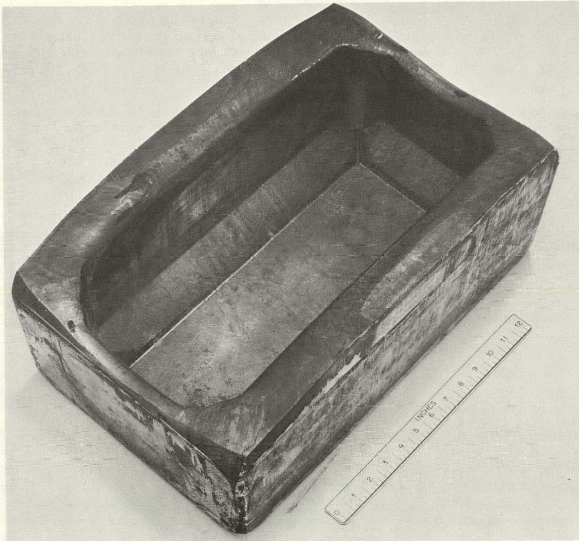
Figure 18. BODY BLANK FOR THE APOLLO LUNAR SAMPLE RETURN CONTAINER.
