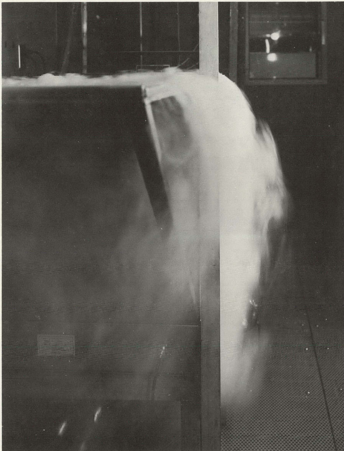
Figure 49. AIR-FLOW CHARACTERISTICS IN A CLASS 100 LAMINAR-FLOW CLEAN ROOM.
