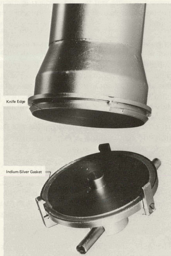
Figure 25. CLOSEUP VIEW OF THE SEALING AREA SHOWING THE KNIFE EDGE AND INDIUM-SILVER GASKET.
