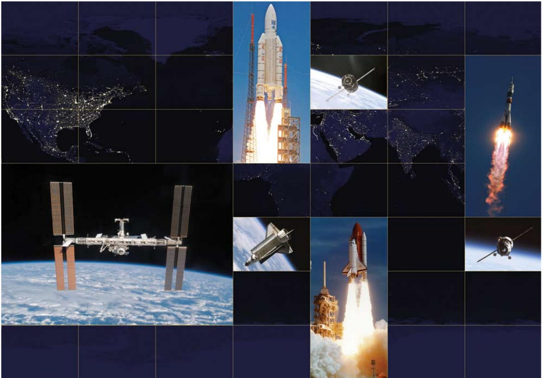
More than 80 flights are scheduled during construction of the International Space Station. These missions deliver equipment, modules, supplies and crew members to the station. The international fleet of vehicles includes the space shuttle (U.S.), Soyuz (Russia),
