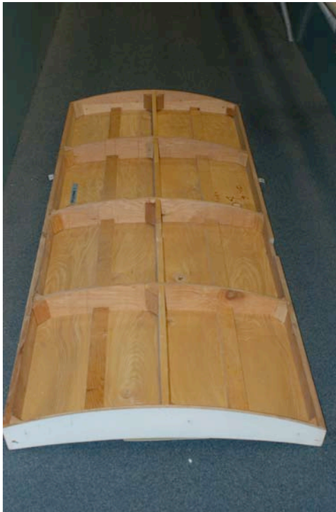
Wood framing and plywood skin of a payload bay panel see from the reverse.
