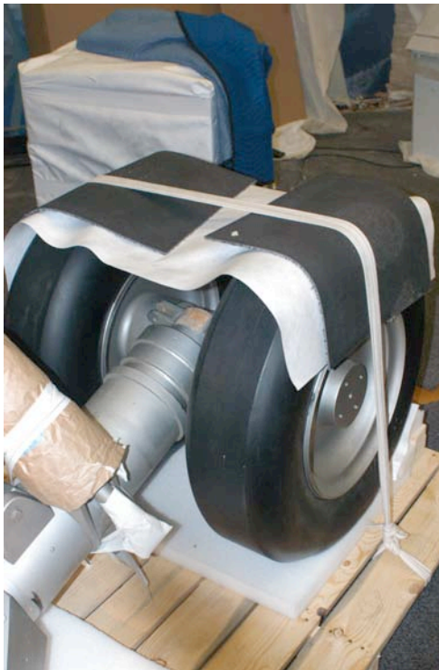
The painted wooden wheels of the nose landing gear padded with Tyvek and braced to the pallet. Ethafoam polyethylene foam planks and wedges were used for additional support.
