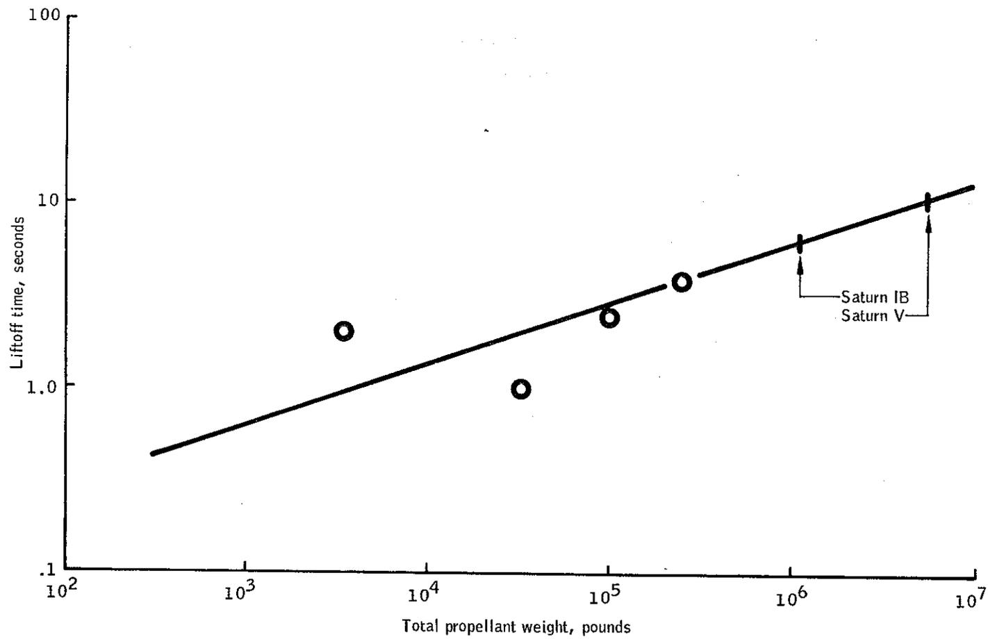
Figure 6.- Fireball liftoff time for various propellant weights
