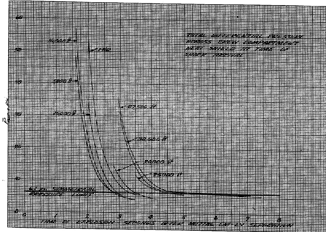
Figure 6.- Total pressure loads - explosion of S-II stage (Saturn V).
