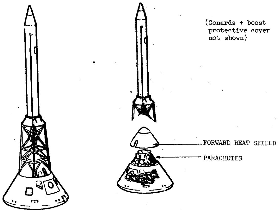
Figure 1.- Forward heat shield deployment.
