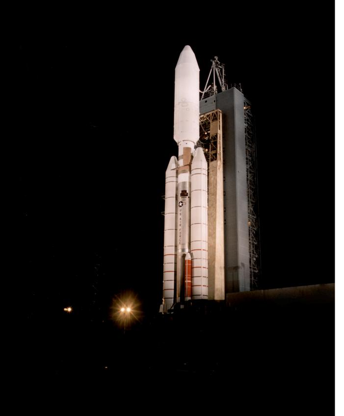
\* Note: 41 seconds after lift-off on 12 August, an electrical malfunction caused the Titan IV A-20 to lose guidance control. The launch vehicle and the payload were destroyed.
