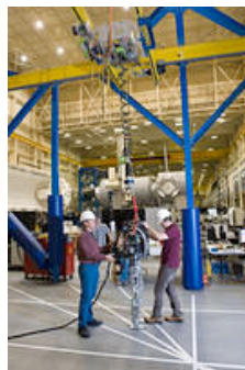
Prototype Legs Walking in Active Response Gravity Offload System
