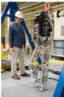
Prototype Legs Walking in Active Response Gravity Offload System
