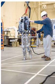
Prototype Legs Walking in Active Response Gravity Offload System
