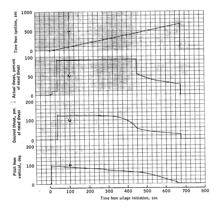
Figure .- Time history of trajectory parameters for one phase guidance case 815.09.
