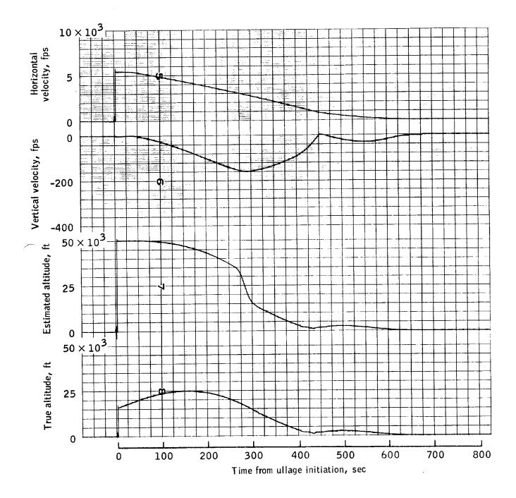
(b) Vertical velocity, horizontal velocity and altitude.
