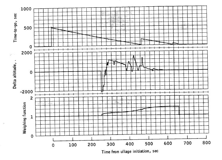
(e) Time-to-go, delta altitude and weighing function.
