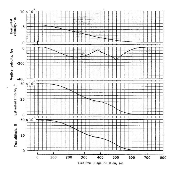
(b) Vertical velocity, horizontal velocity and altitude.
