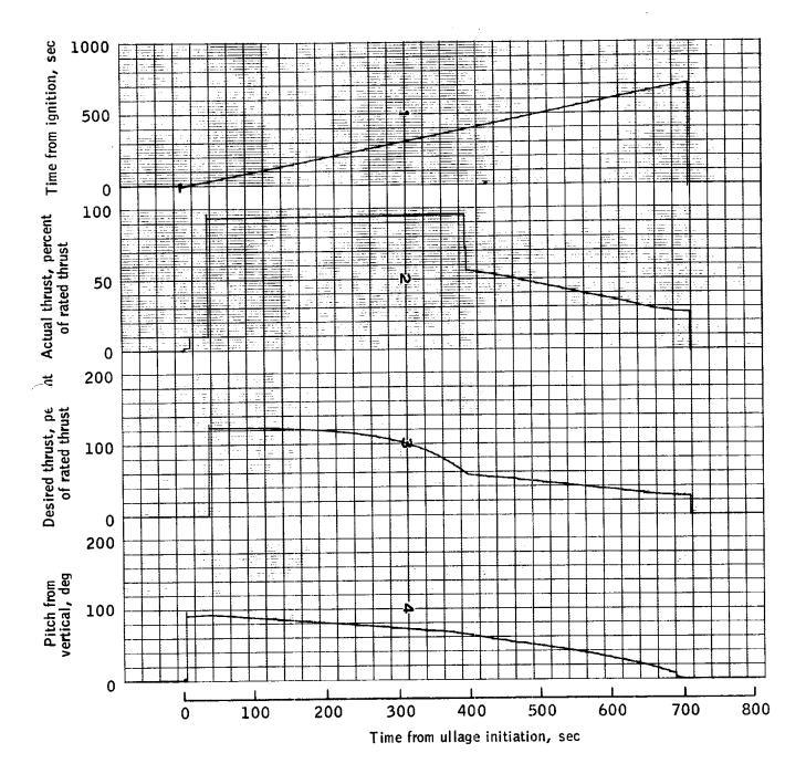
Figure .- Time history of trajectory parameters for one phase guidance case 815.05.
