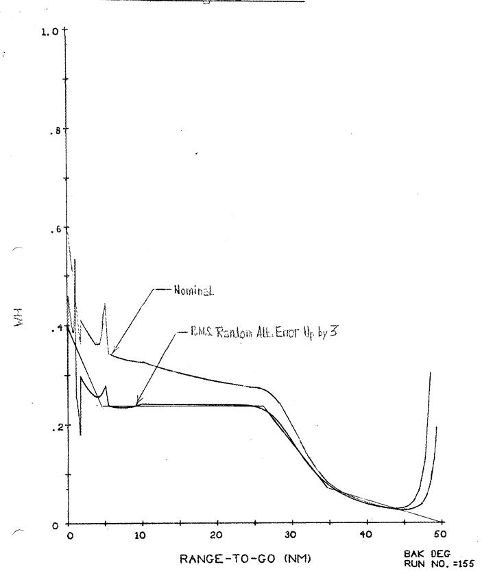
Hy. 12: Effect of Reduced LR Alignment Errors on Velocity Weighting Functions
