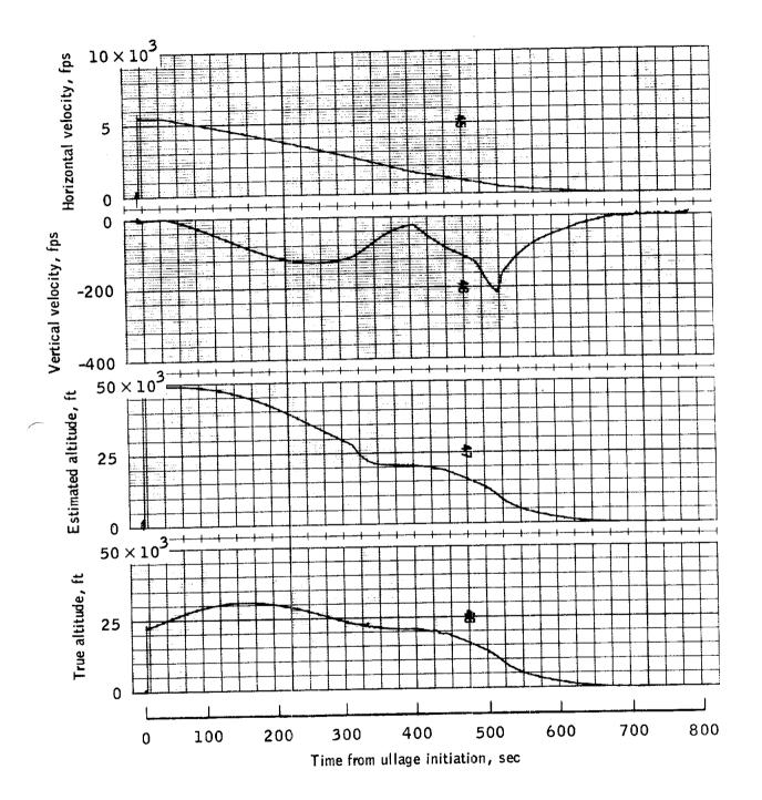
(b) Vertical velocity, horizontal velocity and altitude.
