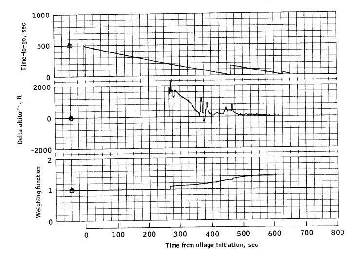
(e) Time-to-go, delta altitude and weighing function.
