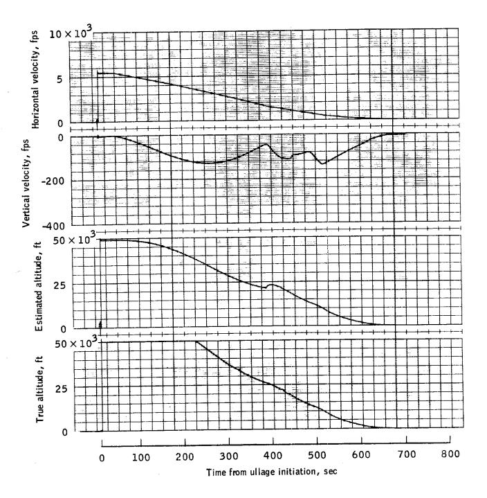
(b) Vertical velocity, horizontal velocity and altitude.
