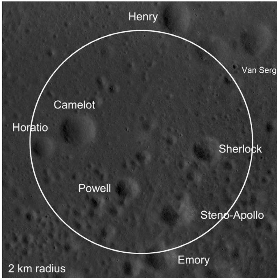
Figure 2: Example of 2.0 km D/L Keep-out Radius at Apollo 17 Taurus-Littrow Landing Site.
