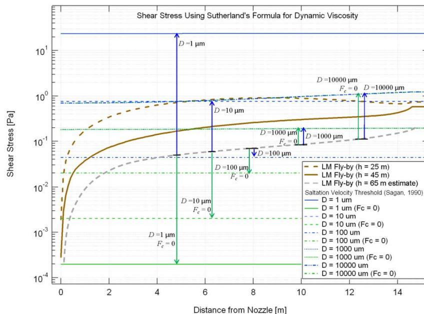
Figure 7: Shear stress generated by a rocket exhaust plume and shear stress levels required to mobilize various sizes of lunar soil particles.
