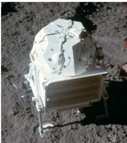
Figure B5 – Solar Wind Spectrometer
