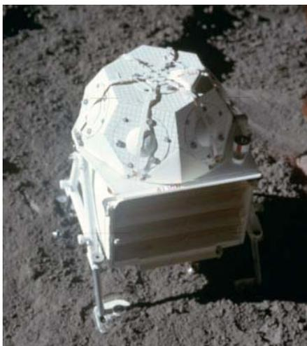
**Figure B5 – Solar Wind Spectrometer**
